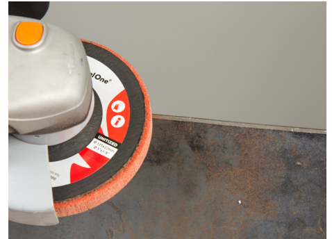
Breaking angles, deburring and rounding.
