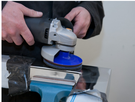
Prepolishing: ideal last step before mirror polishing.
